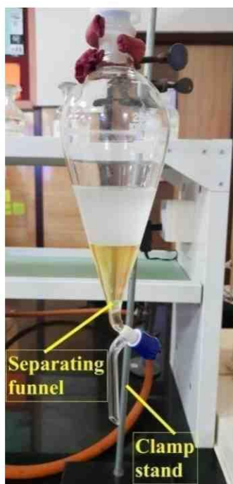
Image 6: Solution after separation of the chloroform layer at the bottom
